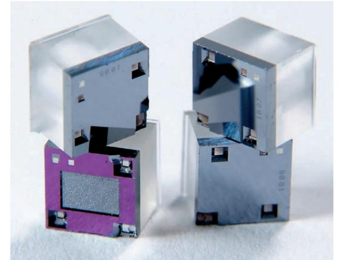
Trench Etched Resonant Pressure Sensor: TERPS
