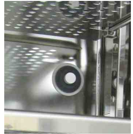
Figure 6. GMP231 probes installed for the incubator test. Outside view (left), inside view (right).
