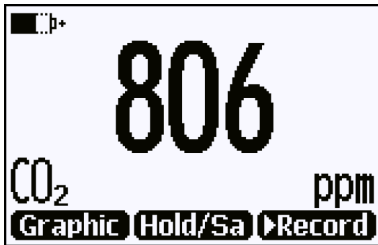
Figure 16 CO 2 reading on MI70 screen
