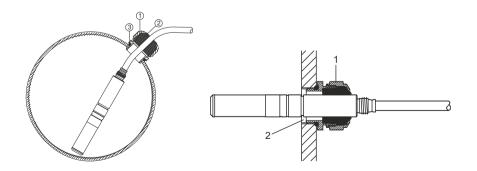
HMP247CG: Vapor-tight installation with cable gland.
