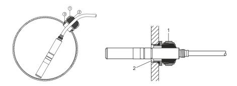
HMP247CG: Vapor-tight installation with cable gland.
