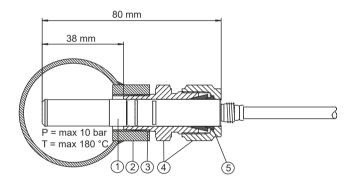
Pressure-tight Swagelok installation kits **SWG12ISO38** with ISO3/8" or **SWG12NPT12** with NPT1/2" thread (SWG6ISO18 with ISO1/8" or SWG6NPT18 with NPT1/8" thread for HMT337 temperature probe).
